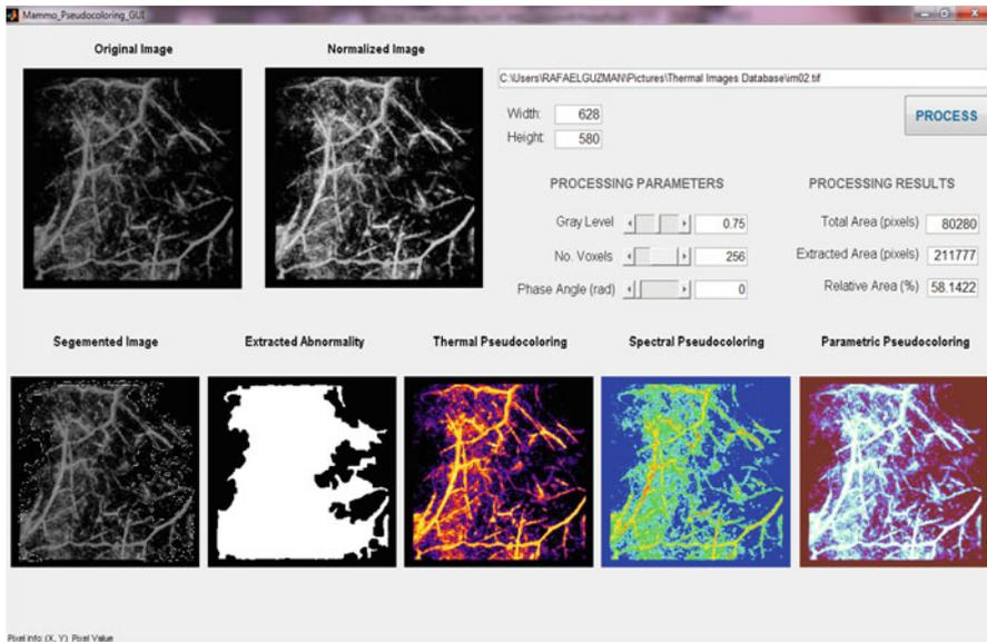
**Fig. 2** Graphical interface of the implemented system to find abnormalities in photoacoustic images
