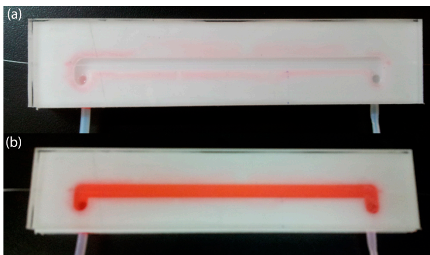
Figure 3. MMI sensor fixed into the Delrin channel with glass cover (a) without gasohol and (b) with gasohol. Red dye is added to the gasohol solution to highlight the gasohol in the channel.
