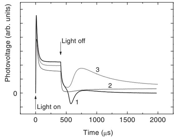
**Figure 4.** Temporal evolution of photovoltage in  $\text{Si}_{0.83}\text{Ge}_{0.17}/\text{Si}$  heterostructure after the light is turned on and off: (1) before US loading, (2) at loading with  $\varepsilon \sim 2 \times 10^{-6}$  and (3) 16 h after US loading. The illumination is achieved with a 835 nm LED. The US frequency is 3.1 MHz.
