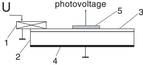
**Figure 2.** Experimental set-up used to excite plate vibrations: 1, piezoceramic transducer; 2, substrate; 3, thin layer; 4, ohmic contact; 5, semitransparent metallic layer.
