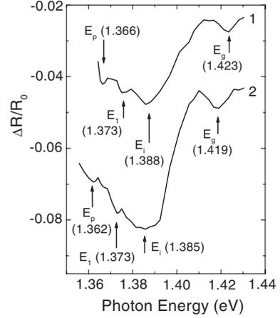
**Figure 6.** Spectral dependence of the relative change in the light reflectivity in GaAs:Te/GaAs caused by acoustic driving at  $U = 18$  V (1) and 24 V (2). The US frequency is 258 kHz.
