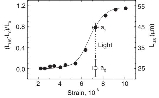
**Figure 3.** Dependence of the diffusion length of minority carriers versus acoustic strain amplitude taken from a Cz-p-Si wafer.  $L_0$  indicates the diffusion length in the absence of acoustic driving while  $L_{us}$  corresponds to that measured at US loading. The value of  $L_0$  is 15–25  $\mu\text{m}$  for different samples. The US frequency is 780 kHz. Points  $a_1$  and  $a_2$  display the data taken in darkness and under light illumination, respectively.
