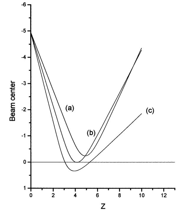
Fig. 5. Position of the beam center as a function of the propagation distance for several values of the incidence angle of the input spatial soliton (a)  $V = 1.1$ , (b)  $V = 1.4$ , (c)  $V = 1.7$ .
