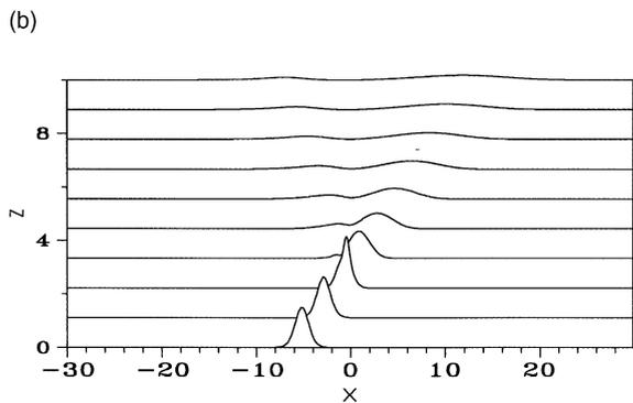
Fig. 4. Reflection and transmission of the bright spatial soliton for an initial incidence angle (a)  $V = 1.7$  and (b)  $V = 2.3$ . The initial energy is splitted into the reflected and transmitted beams, but the reflected beam is still a spatial soliton.
