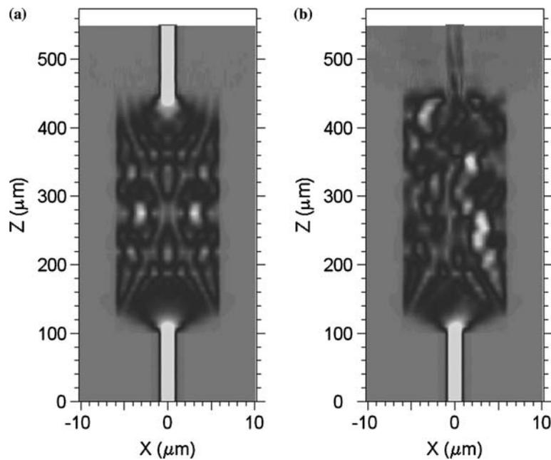
Fig. 2. Beam propagation characteristics (a) Without index modulation, and (b) With an index modulation of  $\Delta n = 1 \times 10^{-2}$ .
