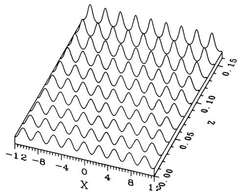
Fig. 4. Numerical result calculated with Eqs. (4) and (5) of modeling the propagation of an interference pattern with 14 fringes/mm through a 9-mm-long BTO crystal. The parameters used were  $T = 1.423$ ,  $\mu = 1$ ,  $R = 25.67$ ,  $a_0 = 0.28$ , and  $b = 20$ .
