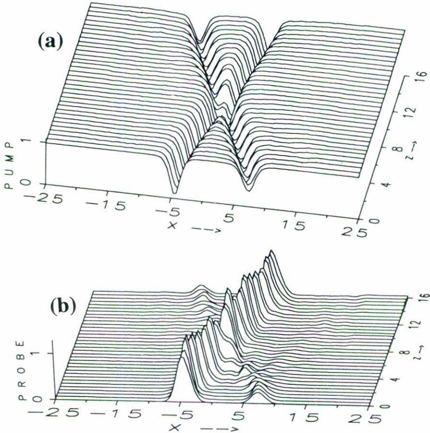
FIGURE 4. The same as in Fig. (3) except that the initial pump profile now consists of two different dark-solitons. Such a profile was taken from Ref. [17] with  $\lambda_1 = -0.3$  and  $\lambda_2 = 0.6$ . Although the asymmetry of the channels, the behavior of the probe beams showed in (b) are essentially the same as in Fig. (3).
