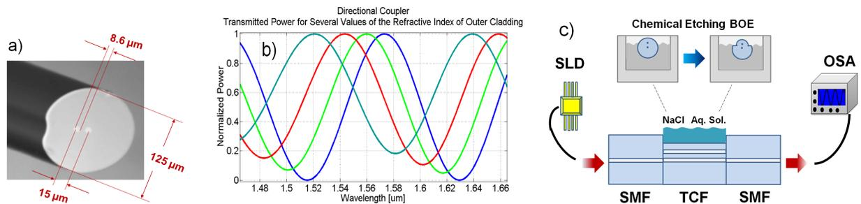
Fig. 1. (a) Cross view of the TCF. (b) Ideal response of the TCF section. (c) Schematic of the TCF RI sensor.
