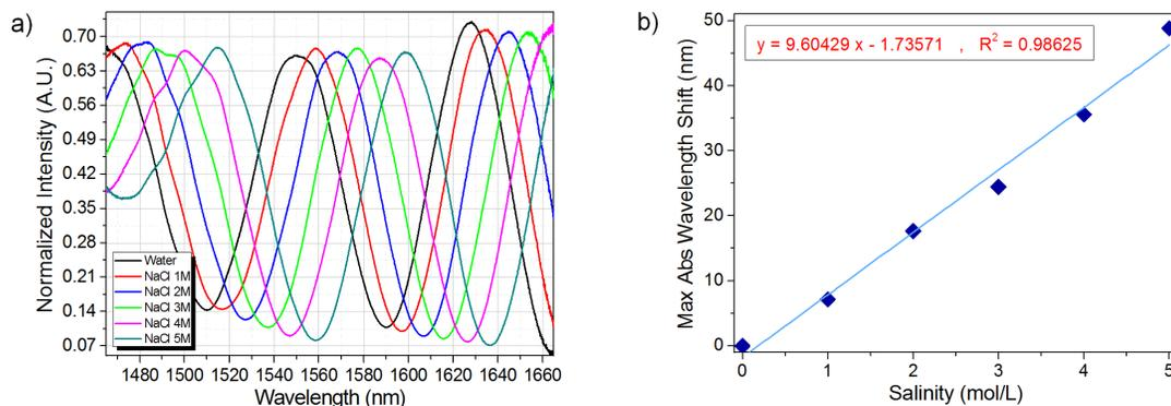
Fig. 2. Response of the TCF salinity sensor in the range from 0 to 5 M. a) Spectral response and b) linear response of the wavelength shift.
