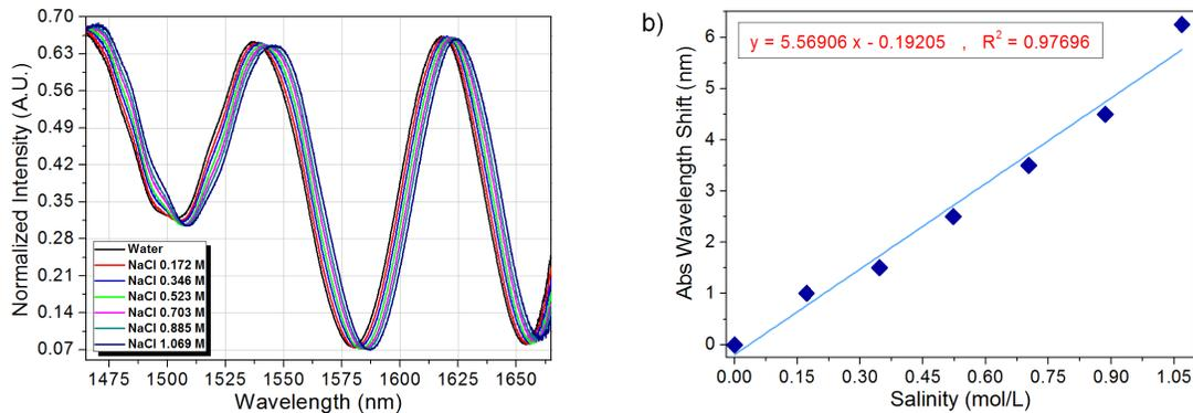
Fig. 3. Response of the TCF salinity sensor in the range from 0 to 1 M. a) Spectral response and b) linear response of the wavelength shift.
