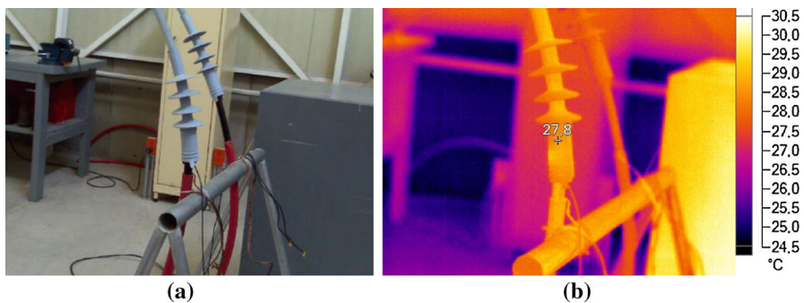
Fig. 9 Pictures of the terminal with failure and partial discharges in two different color palettes: (a) white light and (b) infrared
