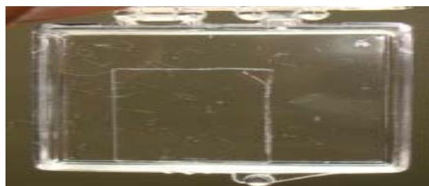
Figure 5 A transparent plastic container with a PDLC sample deposited on a glass substrate (small rectangle).
