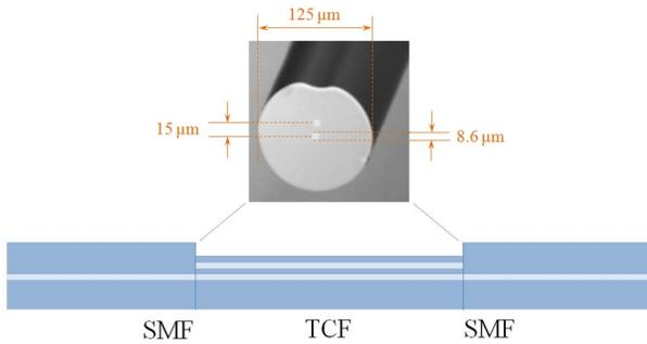
Fig. 1. Schematic of the TCF salinity sensor.
