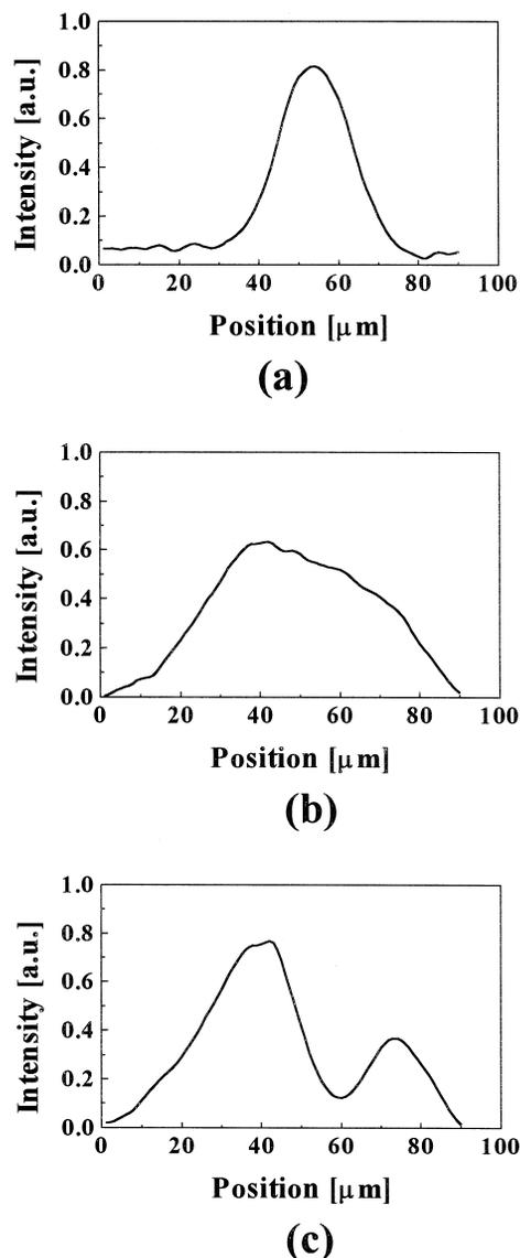
Fig. 6. Profiles for the probe beam: input (a), output (b) and output with 9 kV/cm external electric field applied (c).
