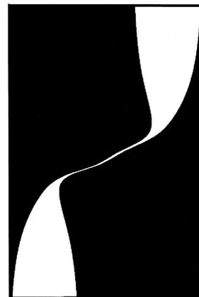
Fig. 3. Unit cell of the computer-generated hologram.
