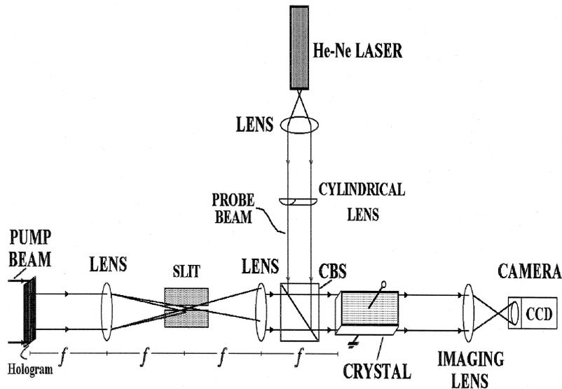
Fig. 4. Experimental set up for the generation of the asymmetric Y-junction. CBS: cube beam splitter.
