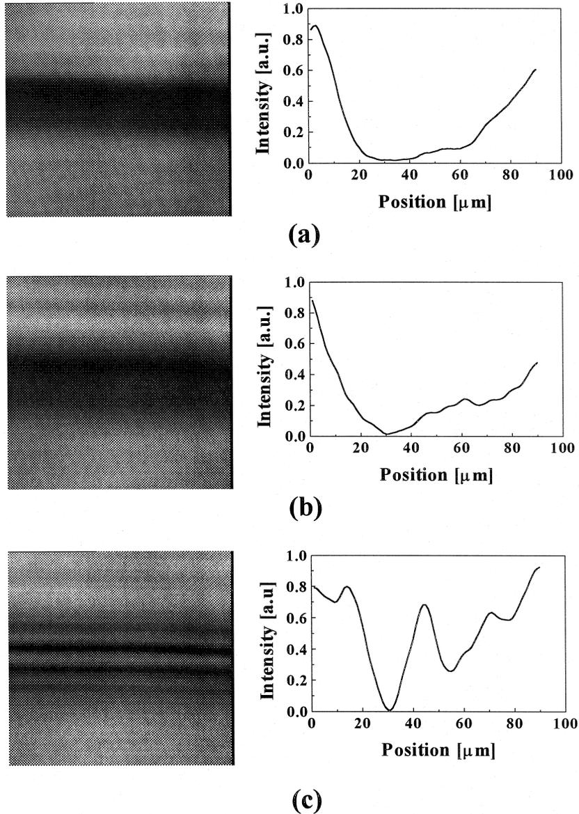
Fig. 5. Images and profiles for the pump beam: input (a), output (b) and output with 9.0 kV/cm external electric field applied (c).
