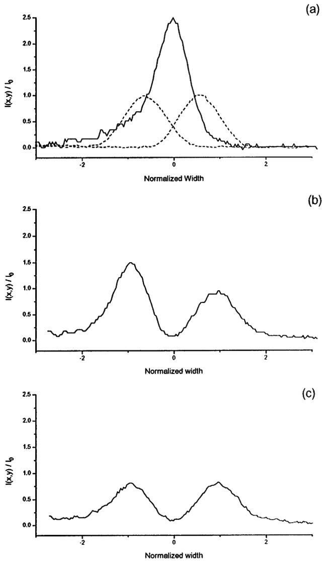
Fig. 2. Experimental output profiles for three values of the relative phase of the initial beams: (a)  $\Delta\phi = 0$ , (b)  $\Delta\phi = 0.65\pi$ , and (c)  $\Delta\phi = \pi$ . The input profiles of the initial beams are graphed with dashed curves in a.
