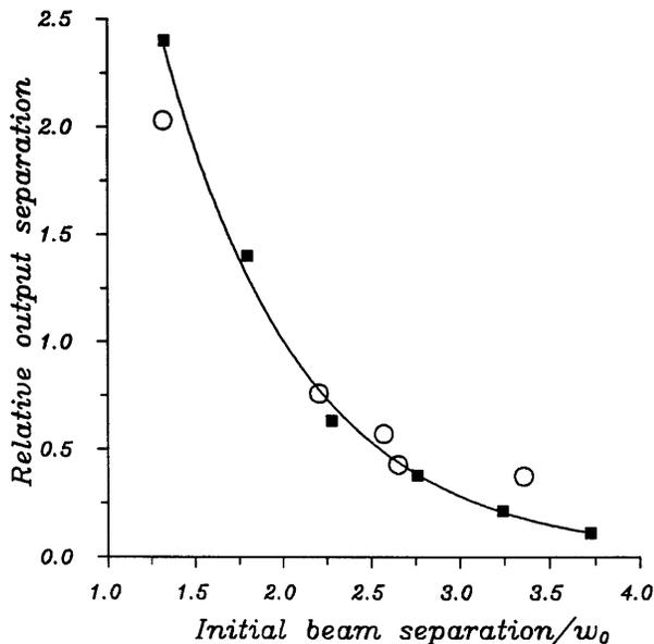
Fig. 4. Relative separation of the output beam with respect to the separation of the input beams as a function of the initial beam separation. Open circles are experimental results, and filled squares are numerical results.
