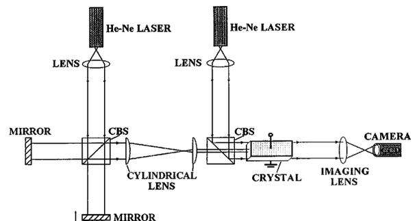
Fig. 1. Experimental setup: CBS's, cube beam splitters.
